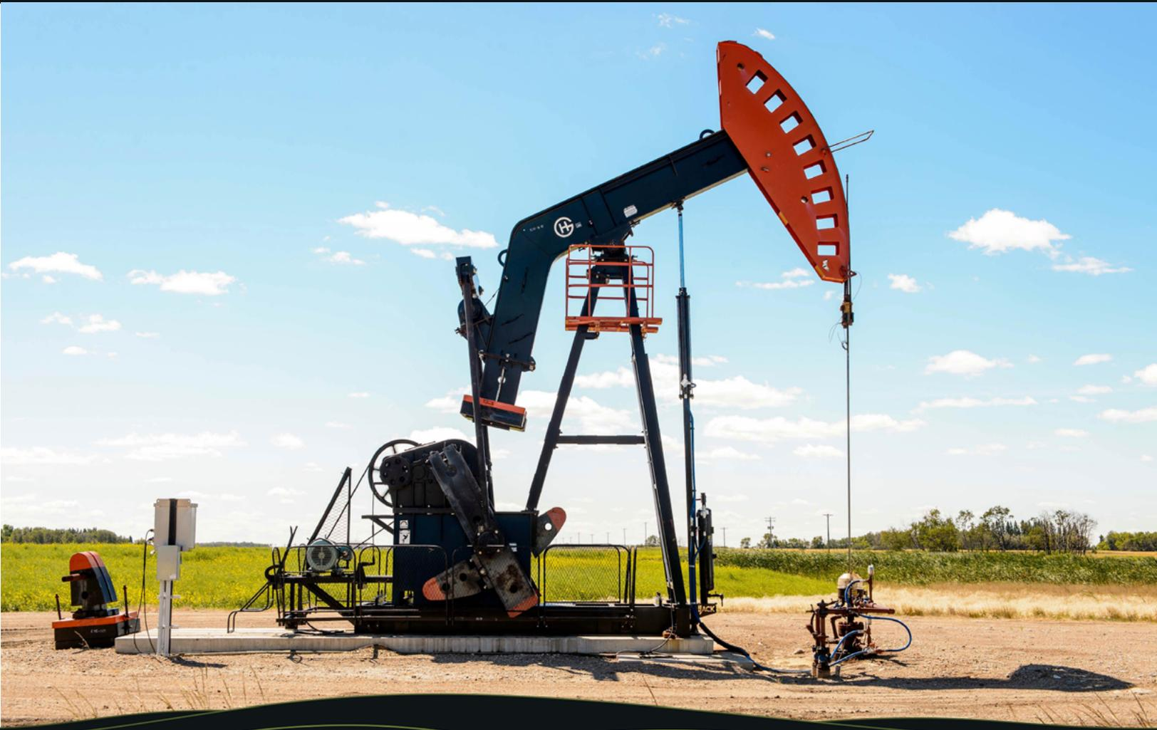
**IJACK DGAS** IS A PRACTICAL AND ECONOMICAL SOLUTION FOR PUMPED OFF / LOW PRESSURE WELLS. BEAM MOUNTED CASING GAS COMPRESSION RELIEVES CASING PRESSURE AND MAXIMIZES PRODUCTION, WHILE ELIMINATING EMISSIONS.
